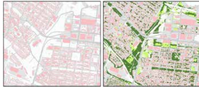
Gray vs Green. Image at left shows an example town’s gray infrastructure including buildings and roads. Classified high-resolution satellite imagery (at right) adds town green infrastructure data layer (trees and other vegetation). The green infrastructure provides cleaner air, water, energy savings and natural beauty.
