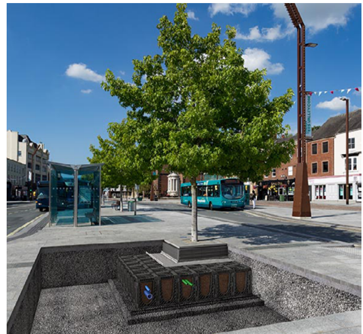
In constrained urban spaces, structural cells can create healthy uncompacted soil volume for urban trees allowing them to grow to their full potential. Image credit: GreenBlue Urban
