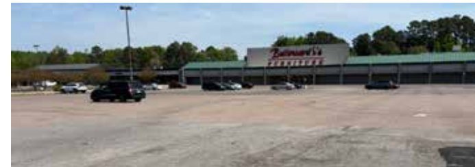
Excess impervious areas cause hotter temperatures and increased runoff. This parking lot could be retrofitted to add more trees, bioswales, and pervious surfaces that allow water to seep into the ground.
