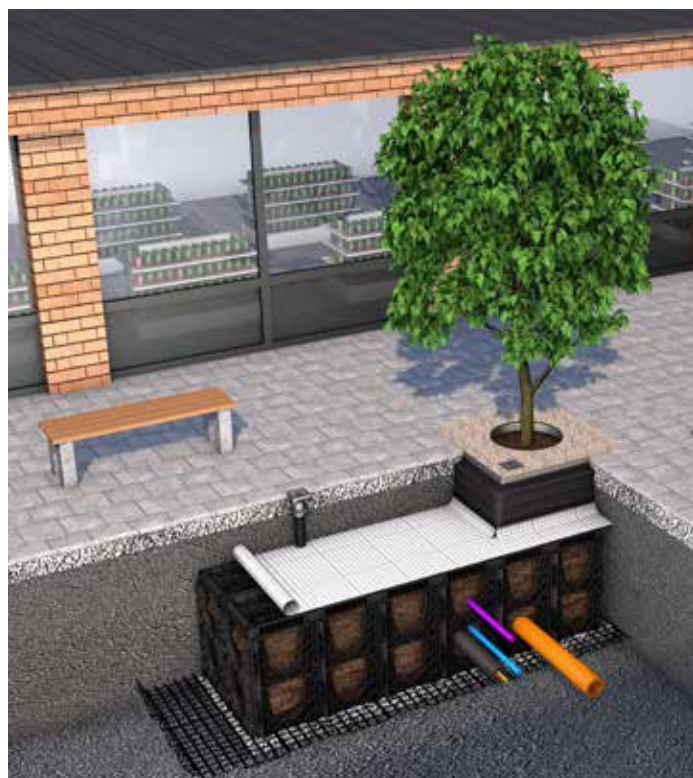
Underground structures can direct roots, and provide space for utilities, allowing large trees and underground utilities to co-exist.
