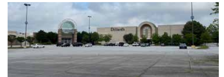
Excess impervious areas cause hotter temperatures and increased runoff. This parking lot could be retrofitted to add more trees, bioswales, and pervious surfaces that let water seep into the ground..
